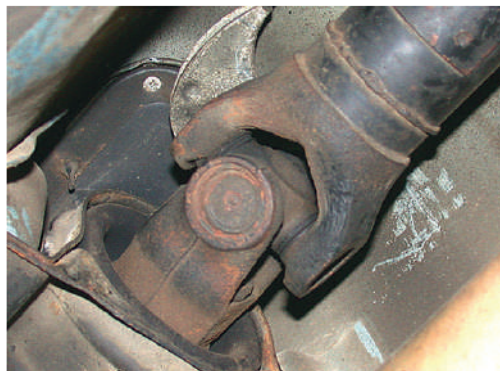
Figure 5.82 Universal joint in position
